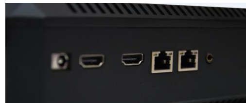
Dual HDMI for Dual Display Mode & Dual LAN for redundancy on Internet Connection
